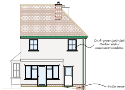
REAR ELEVATION (S) SCALE: 1:100
